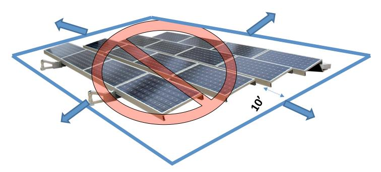
"Conductors more than 5 feet in length inside a building, or more than 10 feet) from a PV array are covered by 690.12"
